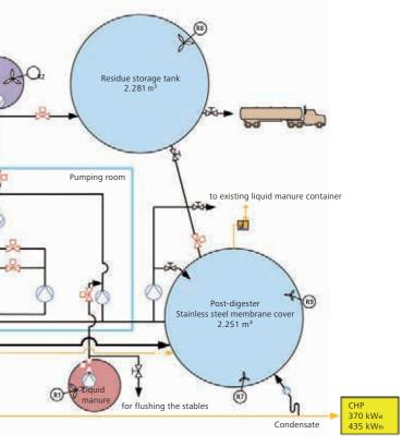
Process scheme biogas plant
