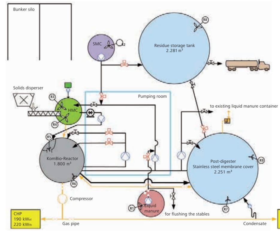
Process scheme biogas plant
