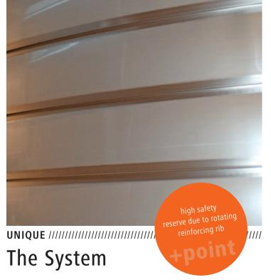
In this system, steel strips are pre-profiled and spirally welded together inside and outside. The root-connected double-welding with molded rotating reinforcing rib on the outside guarantees high stability when picking up static and dynamic loads. The inside of the container, on the other hand, has an edgeless surface. The LIPP-System has proven itself for years and has already been successfully implemented in numerous projects.
